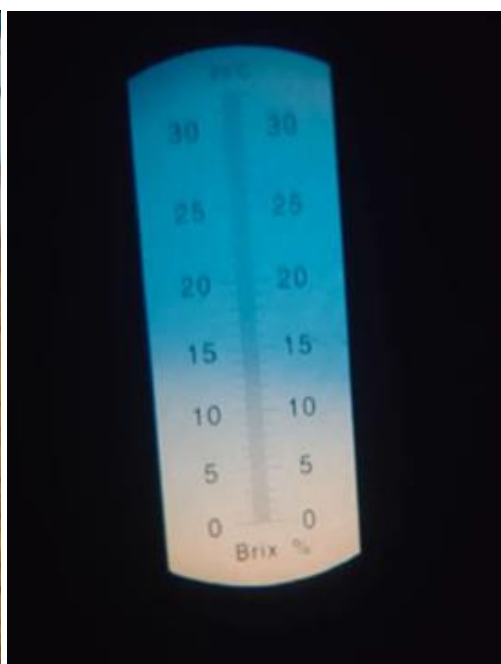
Fig 2: Analysis of Total soluble sugar (TSS) by hand refractometer
