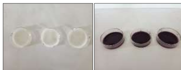
Fig 2: Iodine test for confirmation of extracted starch
